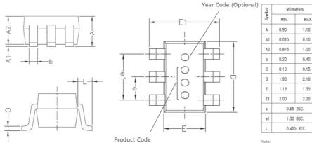
Note: 1.All dimensions are in millimeters, and the dimensions in inches are for reference only. 2.1mm=40mils=0.04inches
